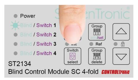
4) Press **Group add/set** button -> Blind 1 (or selected blind) starts flashing (cyan flashing LED indicates group learning mode for the selected blind)
